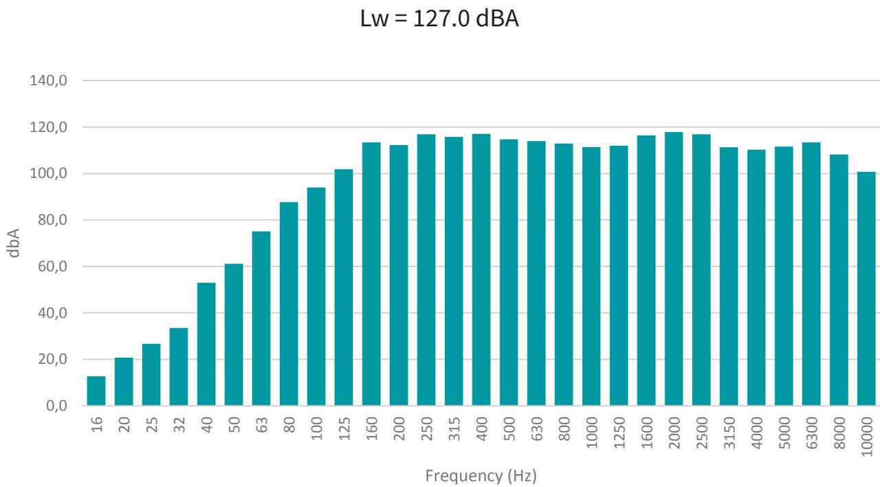
Fig. 4 Sound Power Level Spectrum - 1/3 oct
