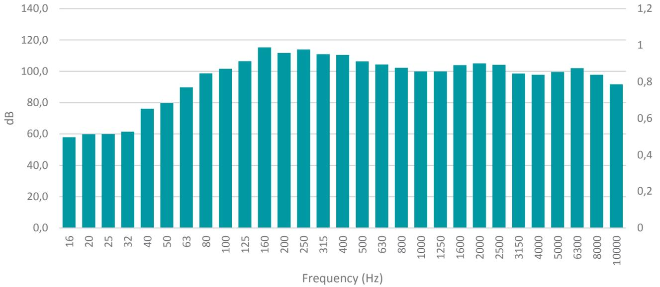
Fig. 5 Linear Sound Pressure Level – 1/3 octave
